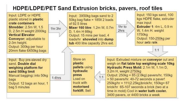
This area should be adjacent to the Brick and Pellet Storage Areas on the output end. It should be adjacent to the Shredding Area and the Sand, Storage, Bagging and Mixing Area on the input side.
